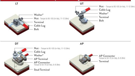
Images shown reflect correct hardware placement. All hardware supplied for AGM with C-max and AES models, motive and solar.
